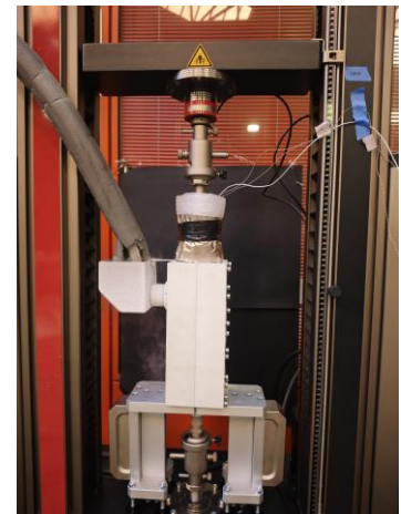
(c) Setup tensile testing with thermal camera for low temperatures
