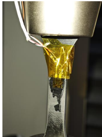
(b) Strain gauge and thermocouple for low temperature
